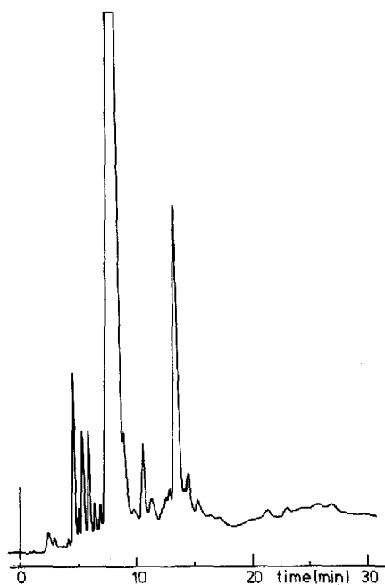
Fig. 10. Separation of three diaminobenzene isomers. Column: 10 cm \times 0.7 cm I.D. (7- \mu m particles, 17-nm pores). Mobile phase: acetonitrile (containing 5% 2-hydroxyethylamine)-water (containing 5% 2-hydroxyethylamine) (30:70), pH 12. Flow-rate: 0.5 ml/min. Detection: 280 nm.
